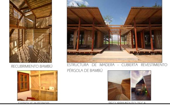
RECUBRIMIENTO BAMBÚ ESTRUCTURA DE MADERA - CUBIERTA REVESTIMIENTO Y PÉRGOLA DE BAMBÚ RECUBRIMIENTO TECA
